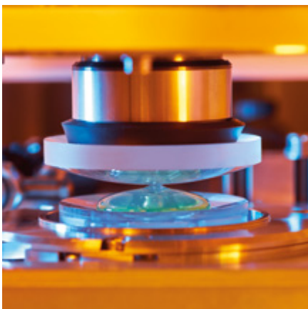
UV adhesive for OPS and OBM Blocking Systems.
