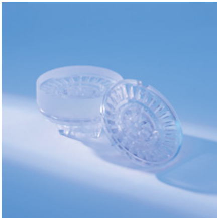
Lens blocked on OBM block with adhesive UV-307A
